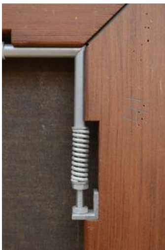
Fig. 1. Corner of an ICA spring stretcher with metal hardware. Image courtesy of Heidi Sobol and Aaron Shugar, October 2021
